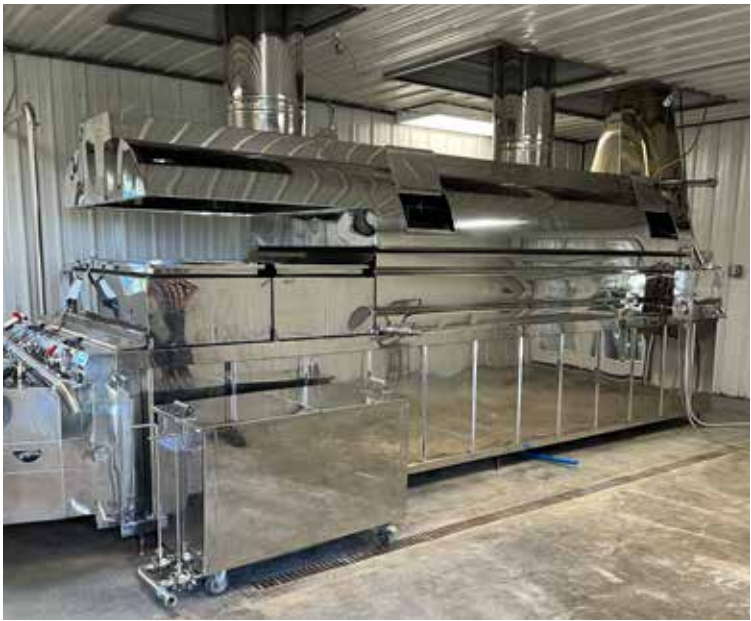
The evaporator is the final concentrating step that uses heat to produce finished maple syrup. Photo by Tommie Kelley
